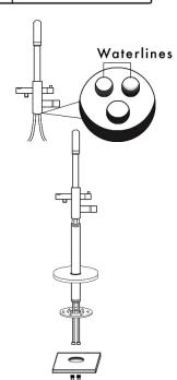
\*Important Note - The Waterlines in the body of the faucet continue 1ft out of the bottom of the body. Please allow space in subfloor installments.
