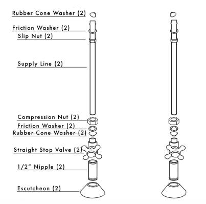
It is always suggested to apply plumber's tape to any threads before installation
